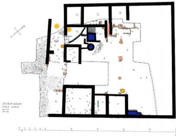
Fig. 6: The vectorisation of the handmade planimetry of the site (author: Flavio Enei). An example of the process that is carried out in IDraw. The superposition of the layer with the original planimetry and the vectorised layer (author: Klára Paclíková).
